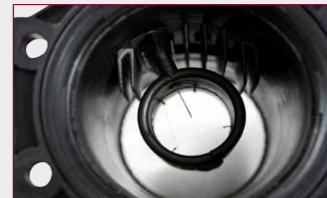
Damage/broken hot wire.
